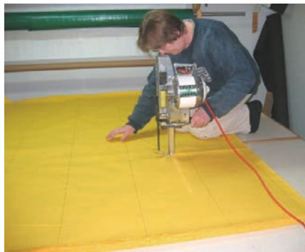
Sandy Smyth cuts layers of canvas with an industrial straight knife
